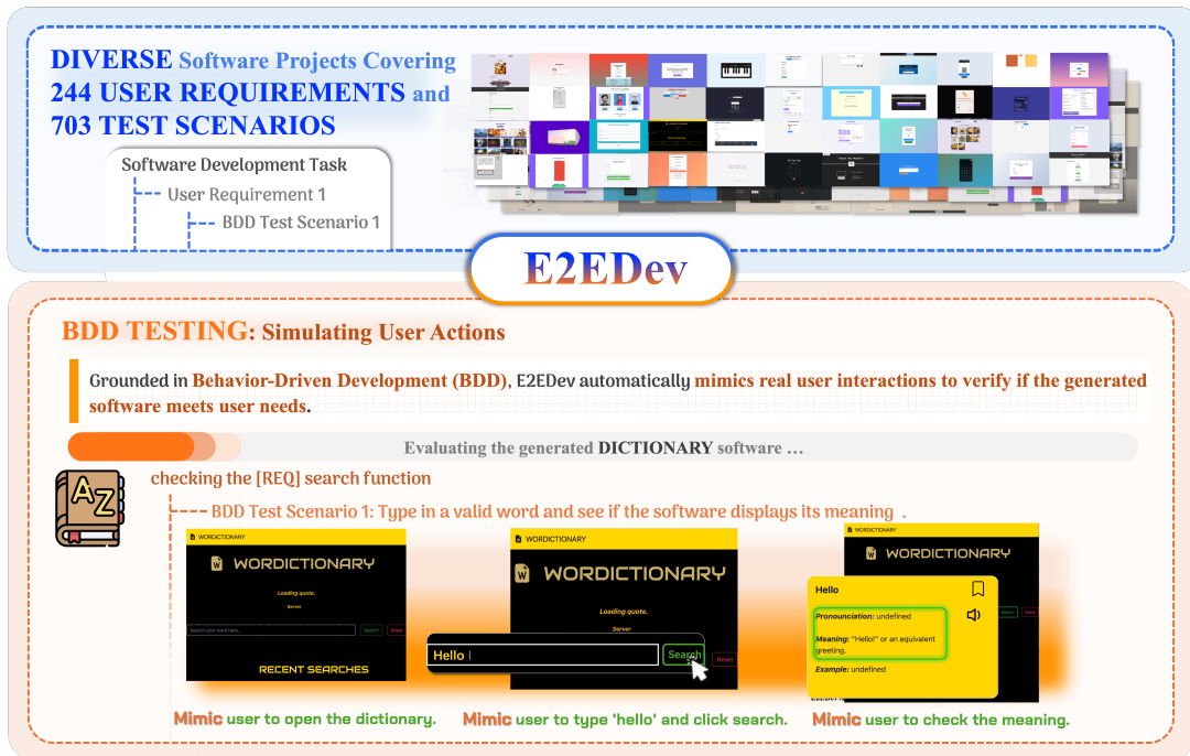
Figure 1: Overview of E2EDev: a dataset and BDD-based automated evaluation pipeline for E2ESD tasks.
