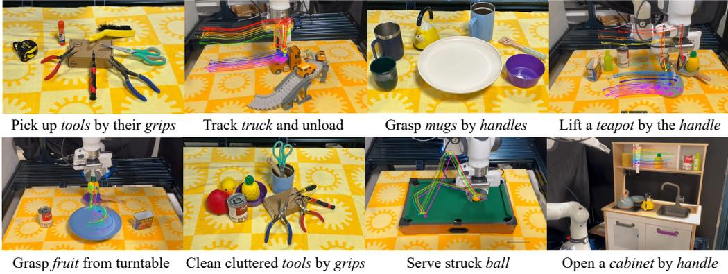
Figure 1: **GraspSplats** supports diverse robotics tasks using feature-enhanced 3D Gaussians. Compared to existing NeRF-based methods [1, 2], GraspSplats transforms the feature representation to reflect object motions in real-time with point tracking from one or more cameras, which makes it possible to perform **zero-shot dynamic and articulated object manipulation by parts**.
