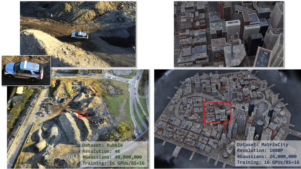
Figure 1: Two large-scale, high-resolution scene reconstructions using Grendel, our distributed 3D Gaussian rendering system. Both images are rendered using 16 GPUs. The left and right images are represented using 40 million and 24 million gaussians respectively. Grendel achieves state of the art quality (PSNR) for both scenes.
