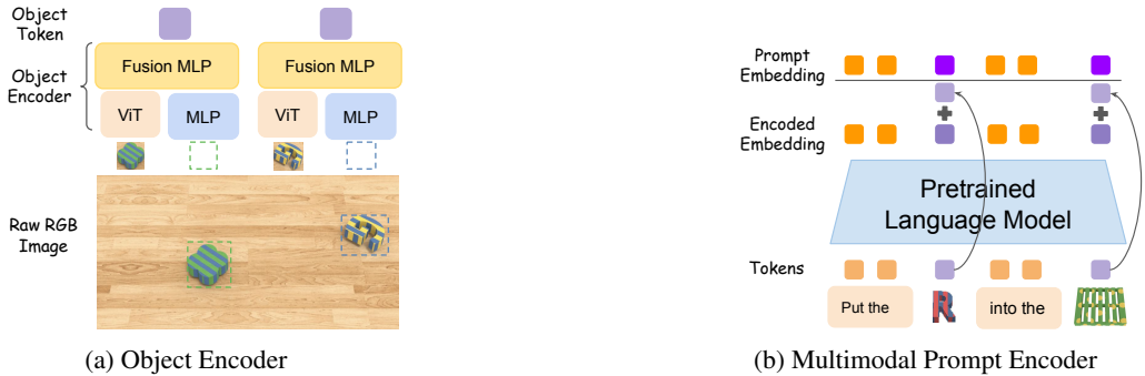
Figure 3: (a) Object Encoder proposed in VIMA consists of a ViT (Dosovitskiy et al., 2020) that extracts visual embedding from cropped object images and a MLP that encodes bounding boxes. The two embeddings are concatenated before passing through a Fusion MLP to get the object tokens. (b) Multimodal Prompt Encoder adds a RC from the input object tokens to the pretrained LM output.
