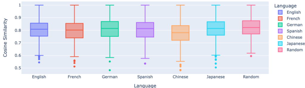
Figure 2: The cosine similarity distributions of RETVec embeddings for 1000 pairs of augmented and non-augmented versions of words, selected languages shown. ‘Random’ language refers to randomly-generated UTF-8 strings.
