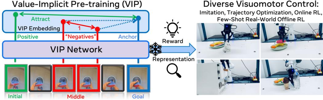
Figure 1: **Value-Implicit Pre-training (VIP)**. Pre-trained on large-scale, in-the-wild human videos, frozen VIP network can provide visual reward and representation for downstream robotics tasks and enable diverse visuomotor control strategies without any task-specific fine-tuning.
