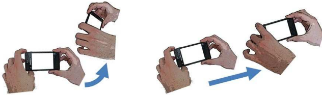
Figure 6. Two possible good motions for SLAM initialization: (left) rotation around a pivot and (right) sideward translation. While the first is an optimal case for the tracker, it is complicated to explain and to perform. The second motion is simpler for a user but still it provides reasonable information to the tracker.
