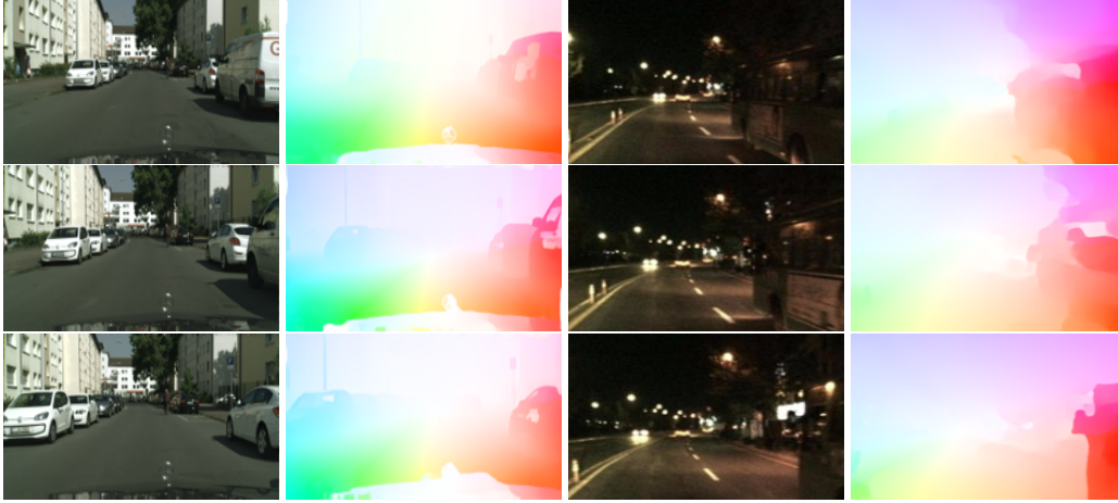
Figure 3: An illustration of optical flows generated using a pretrained FlowNet2 model [27]. The optical flows are generated by utilizing information from the corresponding frame and its previous frame. The left two columns display frames and optical flows under ideal conditions, while the right two columns depict frames and optical flows under adverse weather conditions, with nighttime as an illustrative example. Under ideal conditions, the optical flows accurately capture vehicle details, traffic signs, and poles. In contrast, optical flows under nighttime conditions exhibit significant failures, with missed detection of the middle poles, and erroneous predictions for the bus.
