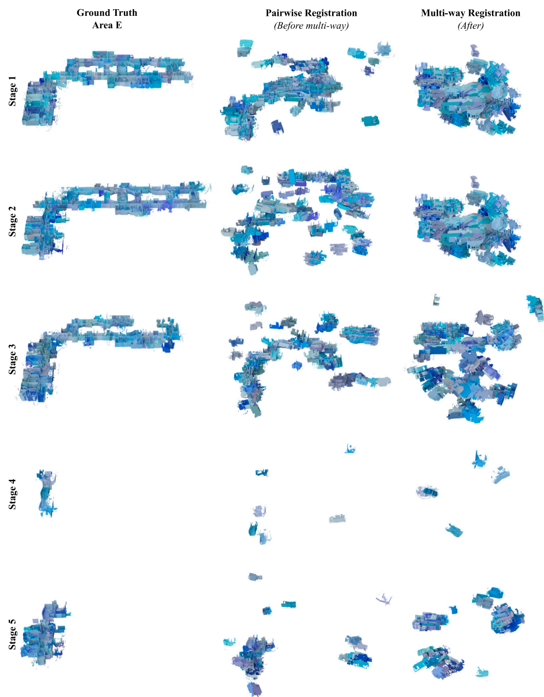
Fig. 25. Spatiotemporal registration results for Area E per temporal stage. Different blue hues denote independent fragment locations. Pairwise registration results from PREDATOR (Huang et al., 2021) and multi-way from Choi et al. (2015).
