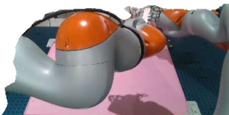
Figure 17: Another example of a problematic data point. The robot pose almost completely occludes the overhead camera's view of the scene, and the color calibration of the wrist and overhead cameras is very different.
