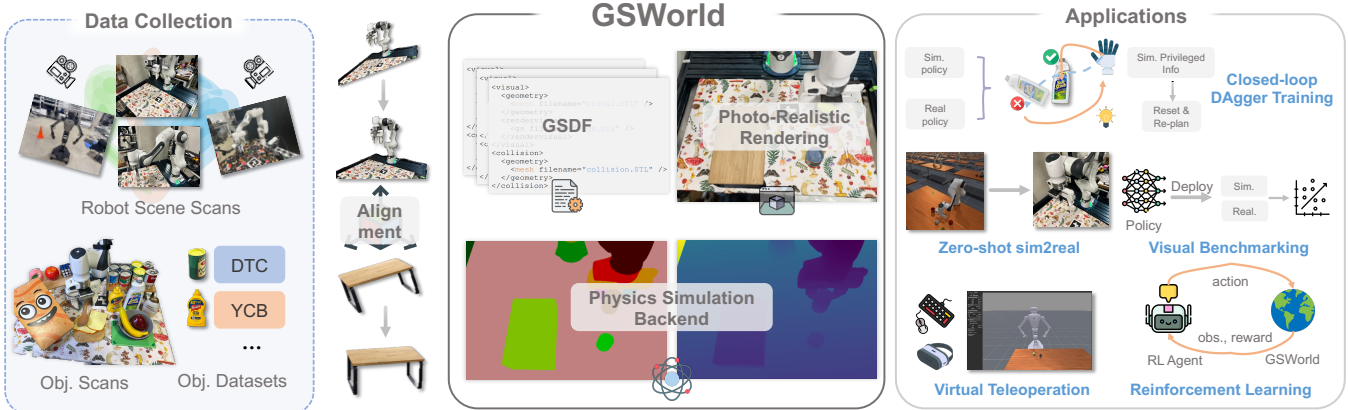
Fig. 2: GSWorld provides an interface on top of existing simulators to render photorealistic assets. Our GSDF assets are compatible with existing simulators to use standard formats for rendering visuals (e.g., depth, segmentation) and computing physics collisions. GSWorld provides a rendering wrapper on top of simulators to make the RGB rendering photo-realistic to support various domain randomization and applications.
