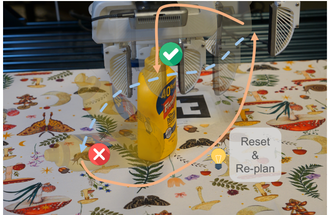
Fig. 3: DAgger Data Collection in Simulation. With privileged information provided by simulation, we can record and relive the failure cases during rollouts and generate corrective data for policy adaptation.
