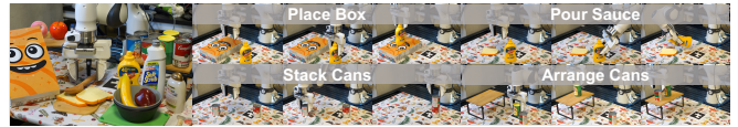
Fig. 5: FR3 Task Visualizations. We design 4 real-world robotic tasks that involve distinct manipulation skills and diverse objects on FR3.
