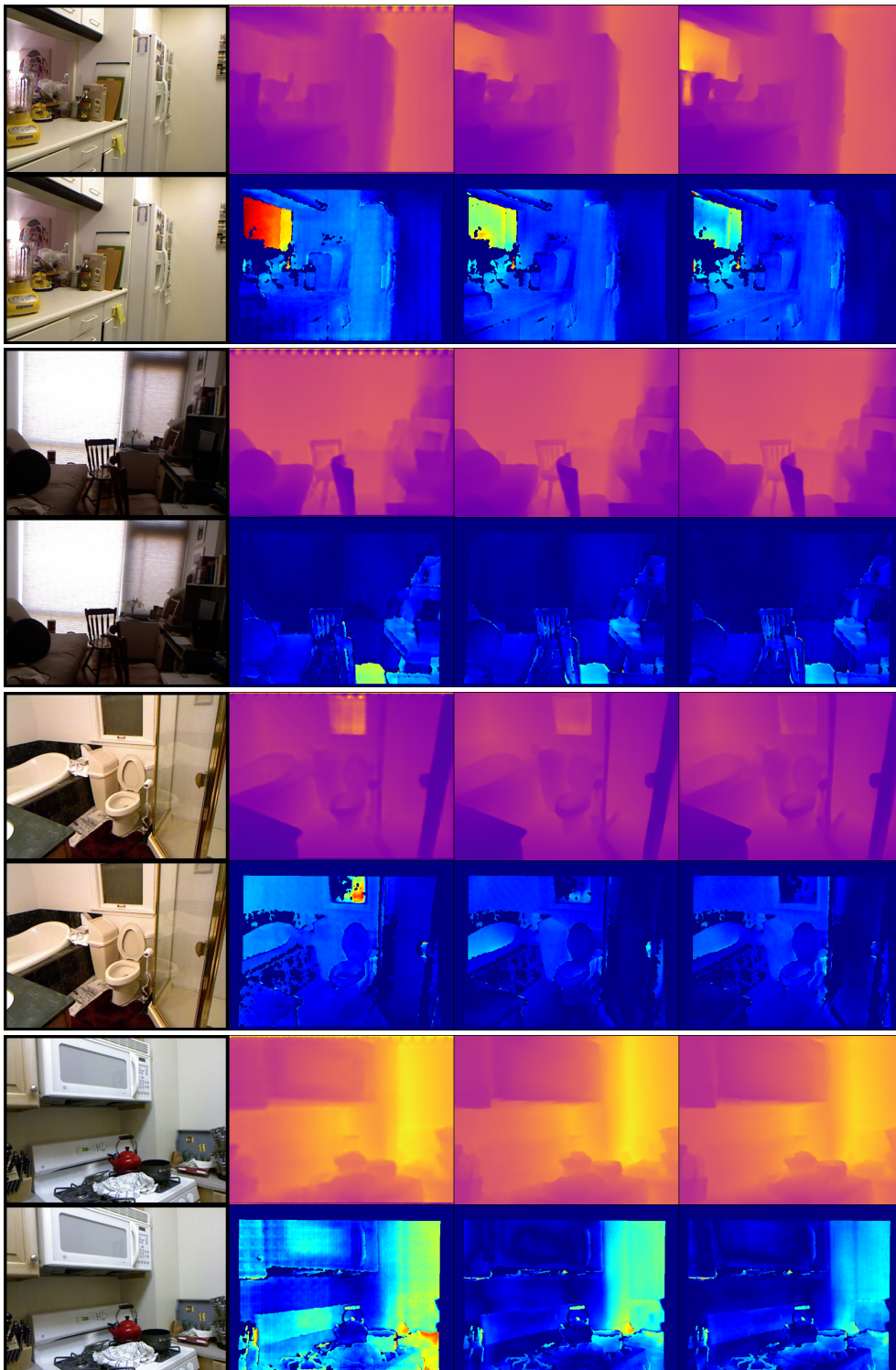
Figure 6: Qualitative comparisons of the three pre-training strategies on NYUv2. Left→right: Image, MP, MP+GP, MP+GP+SP (MeSa). Top : predicted depth maps, bottom : error maps (blue→lower error; red→higher error).
