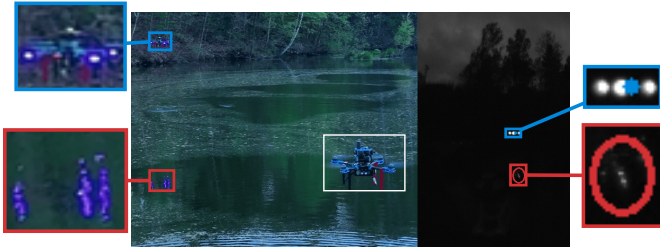
Fig. 5: Outdoor experiment: (Left) Image showing the observing UAV (white), the UAV with the active marker system (blue), and its reflections on the surface (red). (Right) Image captured onboard the UAV using a UV-bandpass filter. The centroid of the UAV equipped with active marker system (blue) and ellipse (red) of the reflection on the water surface.
