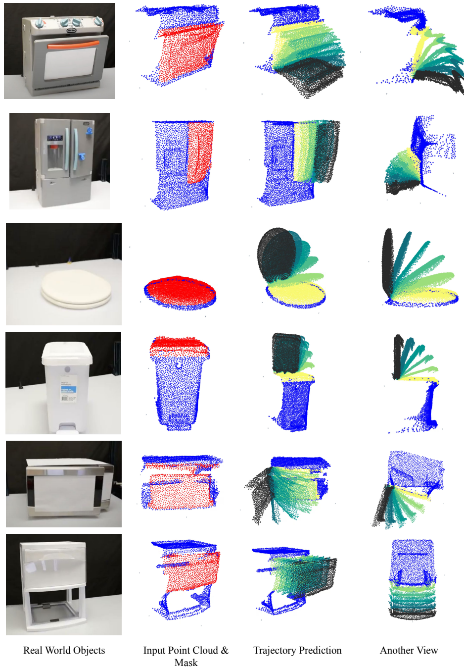
Figure 8: Successful Predictions on 6 Real-World Objects. We show FlowBot++’s prediction quality of 6 different real-world objects. For better readability, we provide an alternative view for each prediction. From top to bottom, the objects are: Oven, Fridge, Toilet, Trashcan, Microwave, and Drawer.
