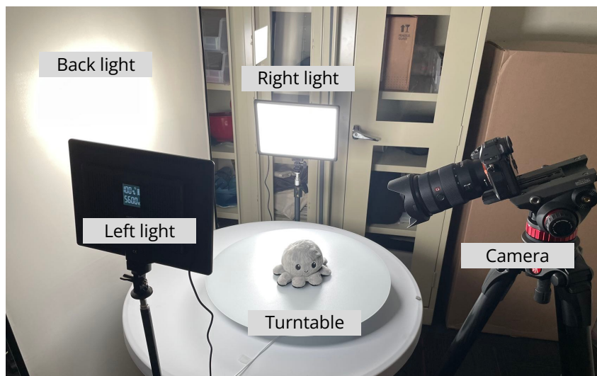
Figure A1: Capture setting for our controlled different illumination and different object poses configurations.
