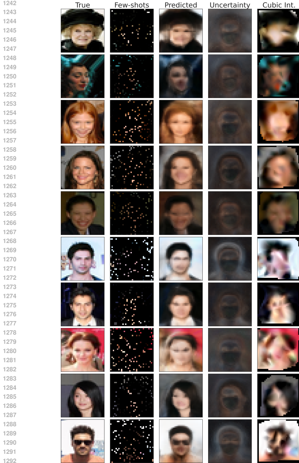
Figure 12: Test-time face completions with NCF* using Taylor order k = 2 , the same order with which uncertainties (variance across 466 candidate predictions) are calculated. This visualization used 100 random pixels.
