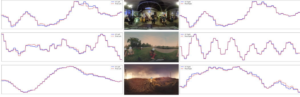
Figure 10: Examples of piecewise signals on YT-Music, ground truth (in blue) and predicted (in red) for the left and right channels.
