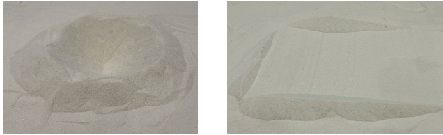
(a) Before (slope = 14.78°) (b) After (slope = 1.44°)
