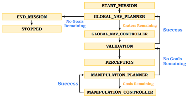
Fig. 2: BEN State Transition Flow
