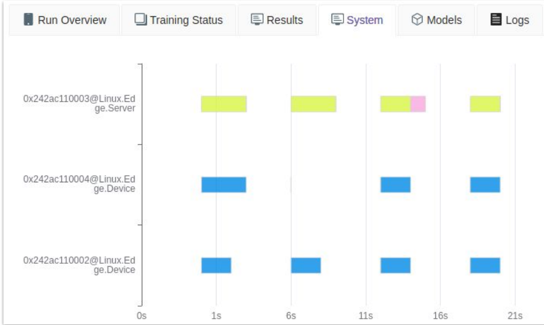
Figure 12: Deployment Interface Example: Overhead distribution monitoring on each edge device (e.g. Desktop (Ubuntu), Laptop (MacBook), and Raspberry Pi 4), which can be used to pinpoint HE overhead bottlenecks and guide optimization.
