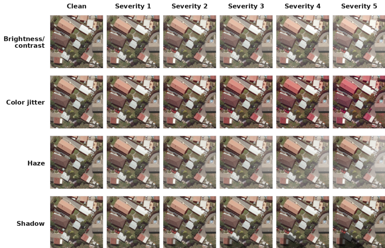
Figure 4. Severity sweep for the pseudo-change perturbations. The same clean WHU-CD [15] patch is shown under brightness/contrast, color jitter, haze, and shadow perturbations. In evaluation, each perturbation is applied to only one temporal image at a time.
