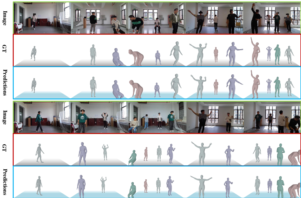
Figure 4: Some 3D Human Mesh Regression Results. We visualize the predicted meshes in three different scenarios, covering the situation of one to four people. The first row is the image captured by the camera, the second row is the ground-truth of the meshes and the third row is the meshes predicted by WiMTR.
