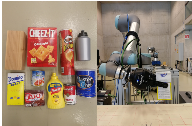
Fig. 4: (left) Object assets used in the real setup. (right) Example of side grasp.
