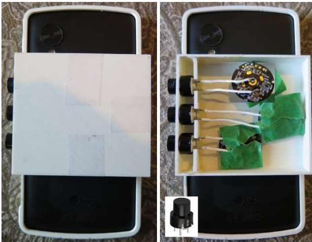
Figure 1: Chording prototype. Left: button housing. Right: Flic Bluetooth PCBs (inset shows pushbutton).
