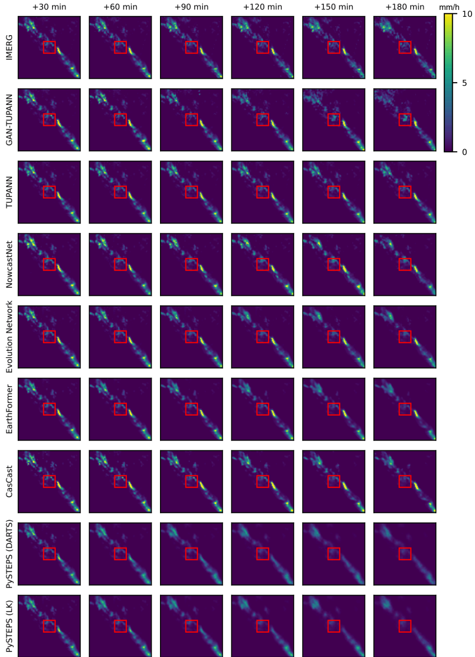
Figure 7: Prediction sample from the IMERG test dataset centered in Rio de Janeiro, starting from 2023-01-08 07:30 UTC. The red square represents the same area as in the GOES-16 figures, demonstrating the difference in spatial resolution.
