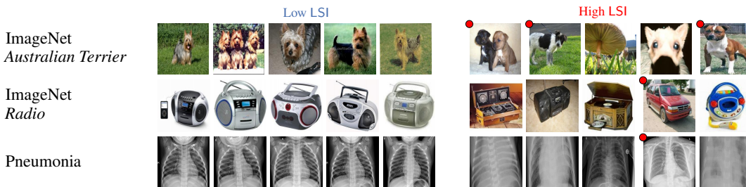
Figure 2: Selected images with low/high LSI in ImageNet and the medical dataset. Samples with low LSI are representative of their underlying class, whereas high LSI samples are often mislabeled/ out-of-distribution (red dots) or atypical with respect to exposure, viewing angle, etc.
