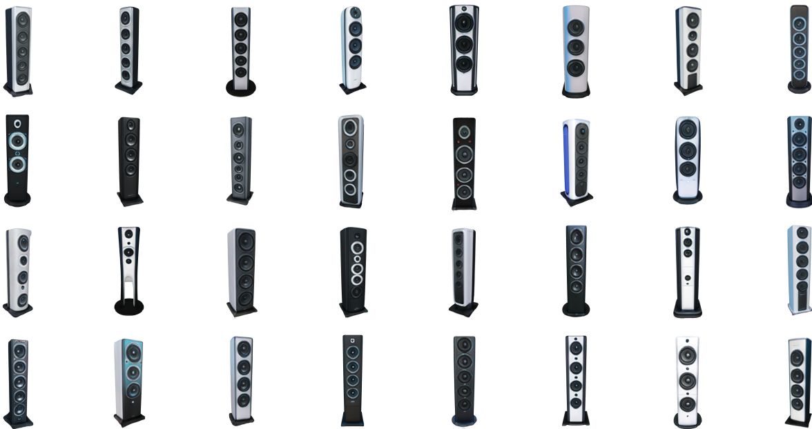
Figure 4. Visualization of the diversity in generated speaker point clouds. We display 32 randomly selected samples from the 120 generated instances. Despite using the same text prompt, varying the random seed results in distinct structural and morphological variations.
