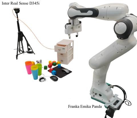
Figure 17: Real-Robot Setup with RealSense D435i and Franka Panda.
