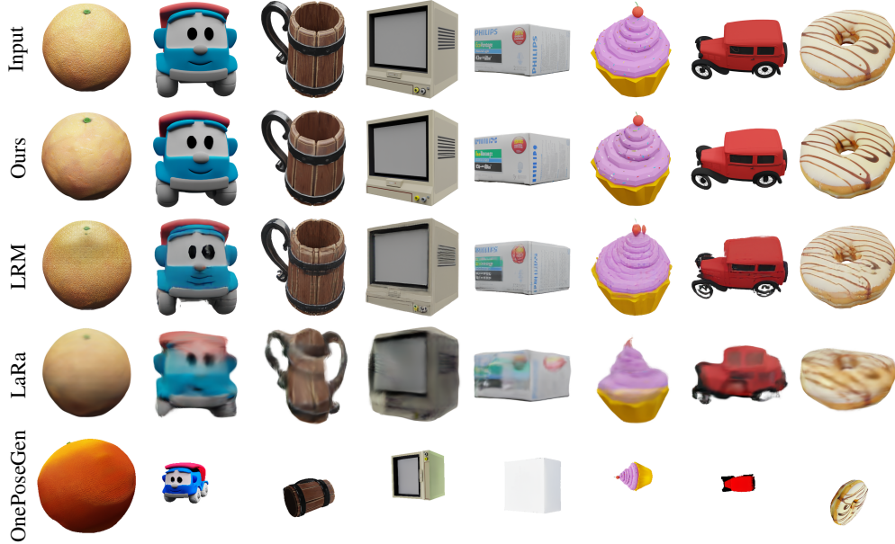
Figure 4: Comparison of generative reconstruction from a single image. Our method produces the highest-fidelity geometry and appearance; LRM hallucinates incorrect details, LaRa is overly blurry due to 2D diffusion inconsistencies, and OnePoseGen frequently fails to register pose reliably.
