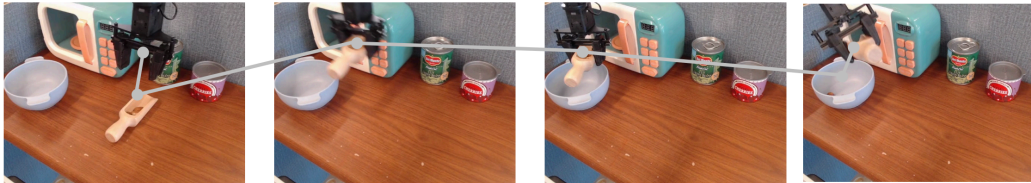
Figure 5: An execution of our method on the task “pour the contents of the scoop into the bowl.” Full breakdown of task and instructions can be seen at Appendix G
