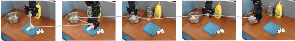
Figure 12: Spatial reasoning failure occurred when masking out low level instruction. The task was to “sweep the mints using the towel.” Due to the presence of the pot and the mushroom, being both strong priors within BridgeData, the policy chose not to follow the high level instruction.
