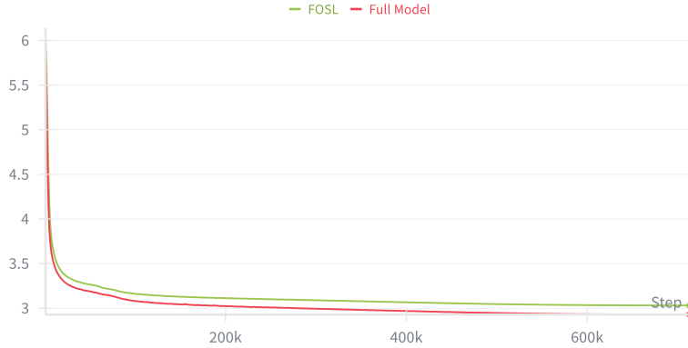
Figure 6: Evaluation loss vs. training step on C4 for LLaMA-130M full-rank and FOSL when trained on a 100B-token budget. FOSL closely follows the dense baseline and ends with a slightly higher but still comparable final loss while using fewer effective parameters and lower memory.
