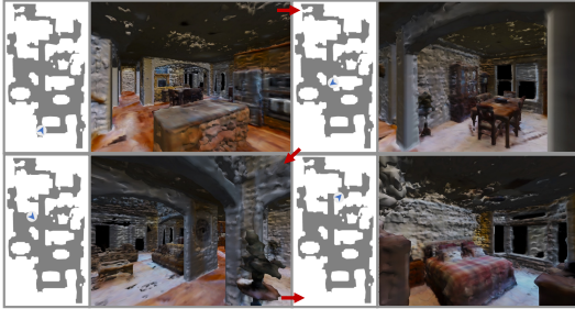
Figure 6: Navigating in the Habitat simulator: the underlying mesh was extracted from the trained NeRF, Ours (cov.) . Rendering quality and the generated BEV map are correct, as are free navigable space and collision handling. Temporal order indicated by \rightarrow .
