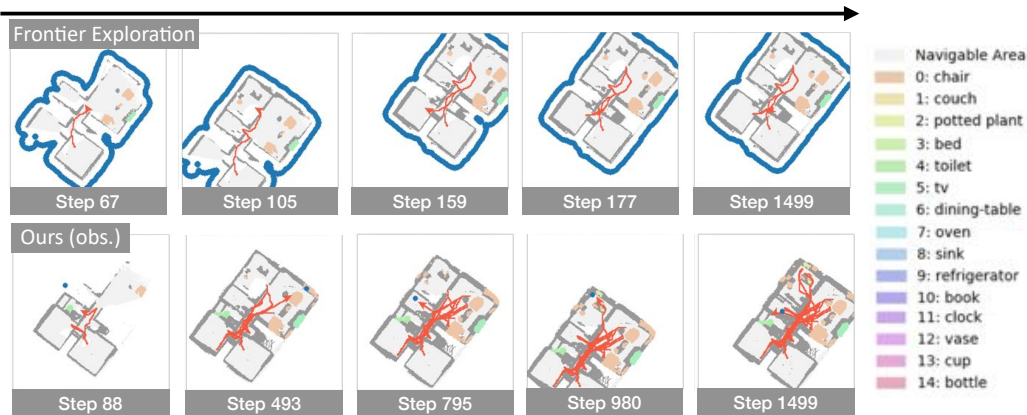
Figure 5: Rollouts by Frontier Based exploration vs. Modular policy ( Ours (obs.) ): FBE properly covers the scene, but does not collect a large diversity of viewpoints, while the modular policy enters the rooms and thus provides richer training data for the neural field.
