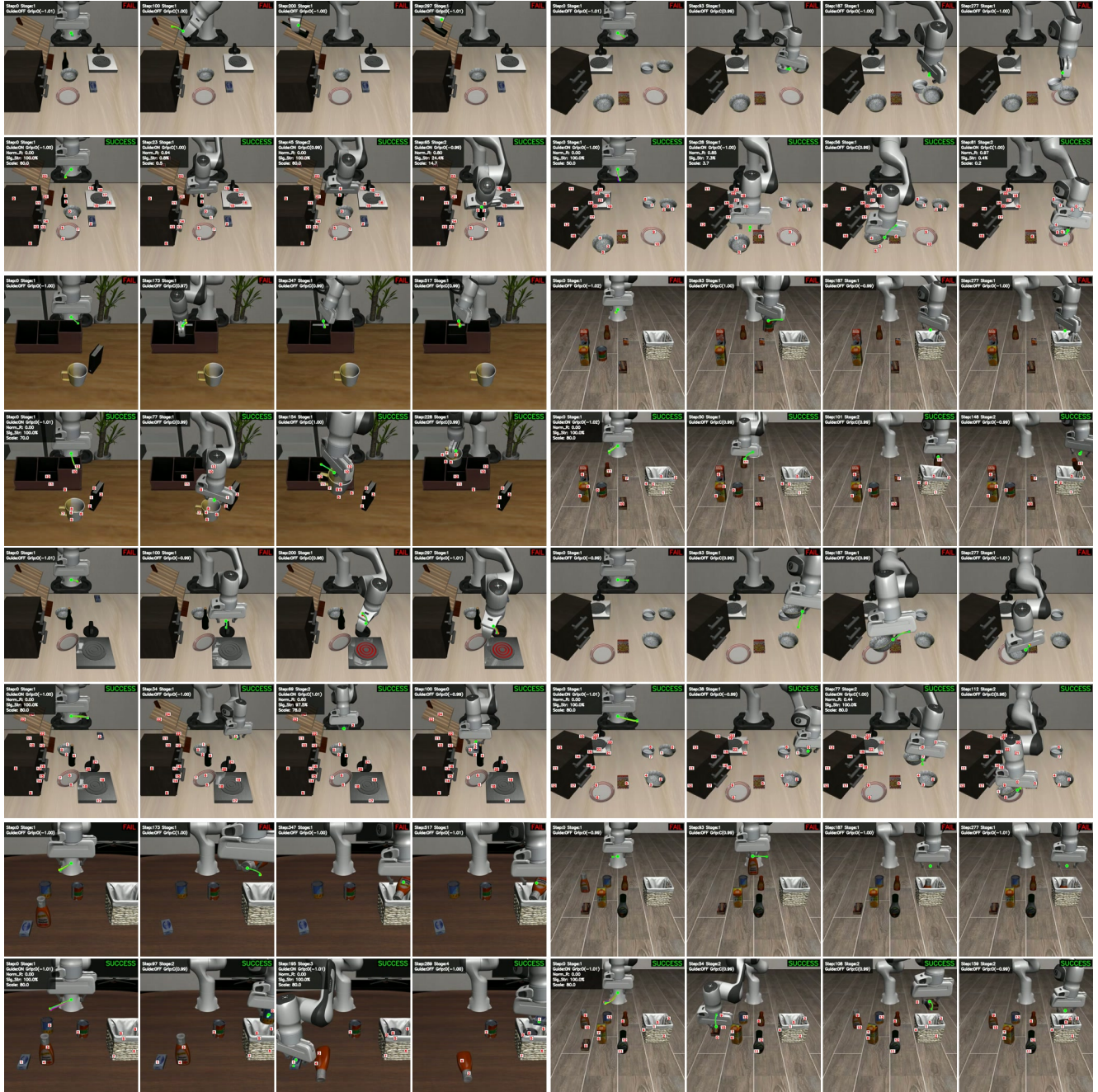
Figure 10. LIBERO-PRO rollouts . Each quadrant compares the base policy (top filmstrip, Fail) with VLS (bottom filmstrip, Success) over four frames. Quadrants (clockwise from top-left): Goal, Spatial, Object, Long-10. Top : Task perturbation (changed language instructions). Bottom : Position perturbation (relocated objects).
