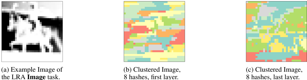
Figure 6: A visualization of learned clusters when using LSHAttention. Here 6a shows the original input image, 6b shows the way pixels are clustered in the first layer of LSHAttention, and 6c shows the way pixels are clustered in the last layer of LSHAttention
