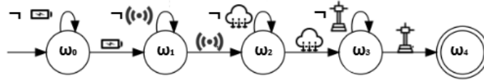
Figure 12: DFA for Mountain Car Collection . The automaton enforces sequential collection of power cell, sensor array, data crystal, and base station return in strict order.
