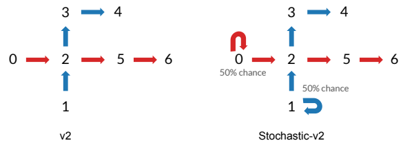
Figure 11: MDP with 7 states and 2 actions (up and right). All episodes end after taking three actions. Data is collected using two policies (red and blue). The only difference between v2 and v2-stochastic, is the data collecting policies are stochastic at states 0 and 1. The stitching task is to navigate from states 0 to 4.
