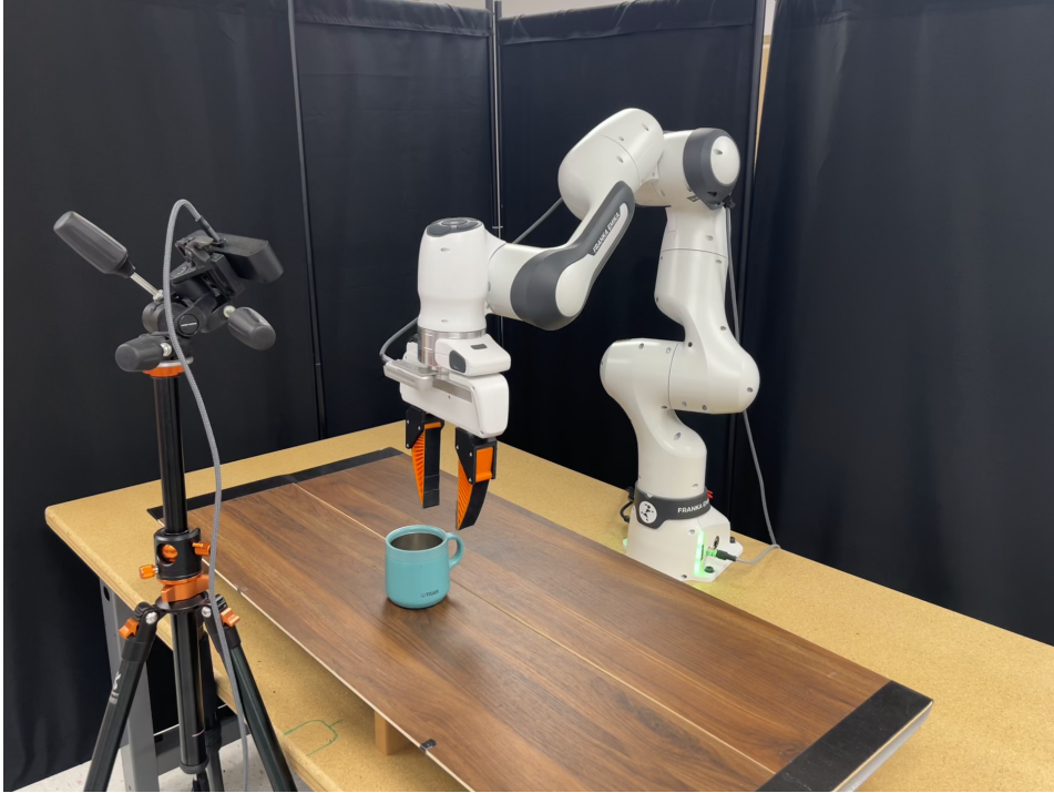
Figure 15: Real Robot Setup. The visualization of the real robot environment and the positions of the cameras.
