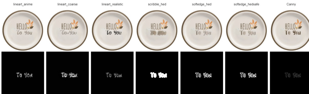
Figure 5: ControlNet Model Evaluation: Canny Edge Detection Prevails Across Varied Conditions
