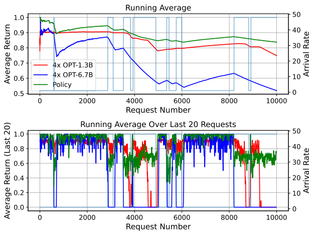
Figure 8: Running total and windowed average over the last 20 requests of performance on the second unpredictable workload. The arrival rate at each step is also shown.
