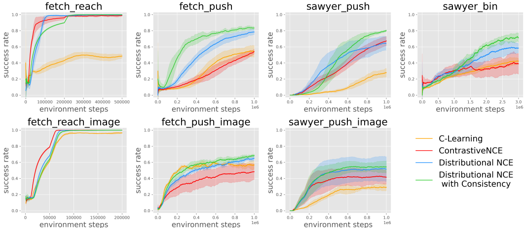
Figure 4: Comparison with baselines. Distributional NCE outperforms the Contrastive NCE (Eysenbach et al., 2022) and C-Learning (Eysenbach et al., 2020) in all but the easiest tasks (fetch_reach, fetch_reach_image). Applying temporal consistency on top of Distributional NCE accelerates learning and boosts asymptotic performance. More comparisons with prior GCRL baselines can be found in Appendix D.1.
