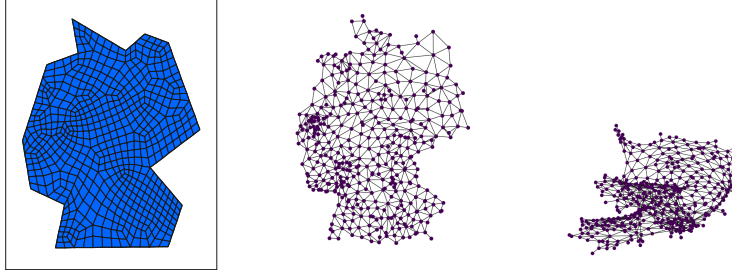
Figure 1: The mesh on the domain for the SI-diffusion equation and the Advection-diffusion equation (left). Independent of this mesh, we build a Graph using administrative regions ( NUTS-3 ), their adjacencies, and the distances of the centers (center). Note, that we used the underlying geo-coordinates to plot this graph (center), while the later used and constructed graph has no trivial unique representation (right).
