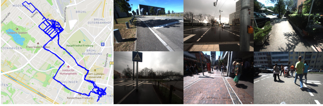
Figure 3: Ego-trajectories (left, blue color) and camera images from our Freiburg Pedestrian Scenes dataset. The dataset features a wide range of urban environments including busy streets, pedestrian areas, and road crossings with varying weather conditions.
