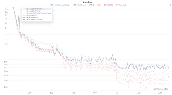
Figure 6: Training loss curves for gradient merging candidates compared with the SFT baseline. The {ATTN} strategy avoids training spikes, while other candidates show instability before convergence.
