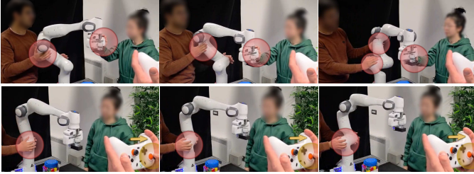
Fig. 4: Non-prehensile Manipulation in Multi-Modal pHRI. Top: Whole-body physical contact compliance. Bottom: Multi-modal pHRI. HANDLE integrates teleoperation, reactive avoidance, and physical contact, enabling robust disturbance rejection under simultaneous interaction. Yellow arrows indicate teleoperation commands.
