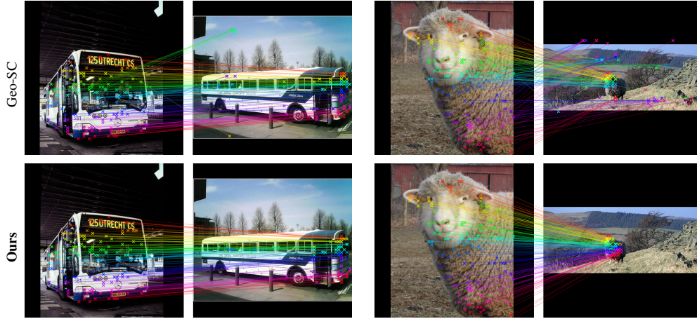
Figure 5: Visualization of keypoint matches for randomly selected object points. On each source image (left) we randomly sample points on the object of interest and compute their match on the target (right). Colored lines are used as a way to distinguish the points.
