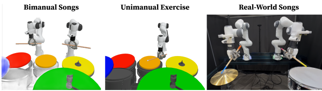
Fig. 5. Drumming Environments. Our first simulation environment includes bimanual, multi-drum song-playing. Our second environment involves unimanual, uni-drum control for a high-speed technical exercise. Finally, in the real-world, we play songs with a drum pad and cymbal.
