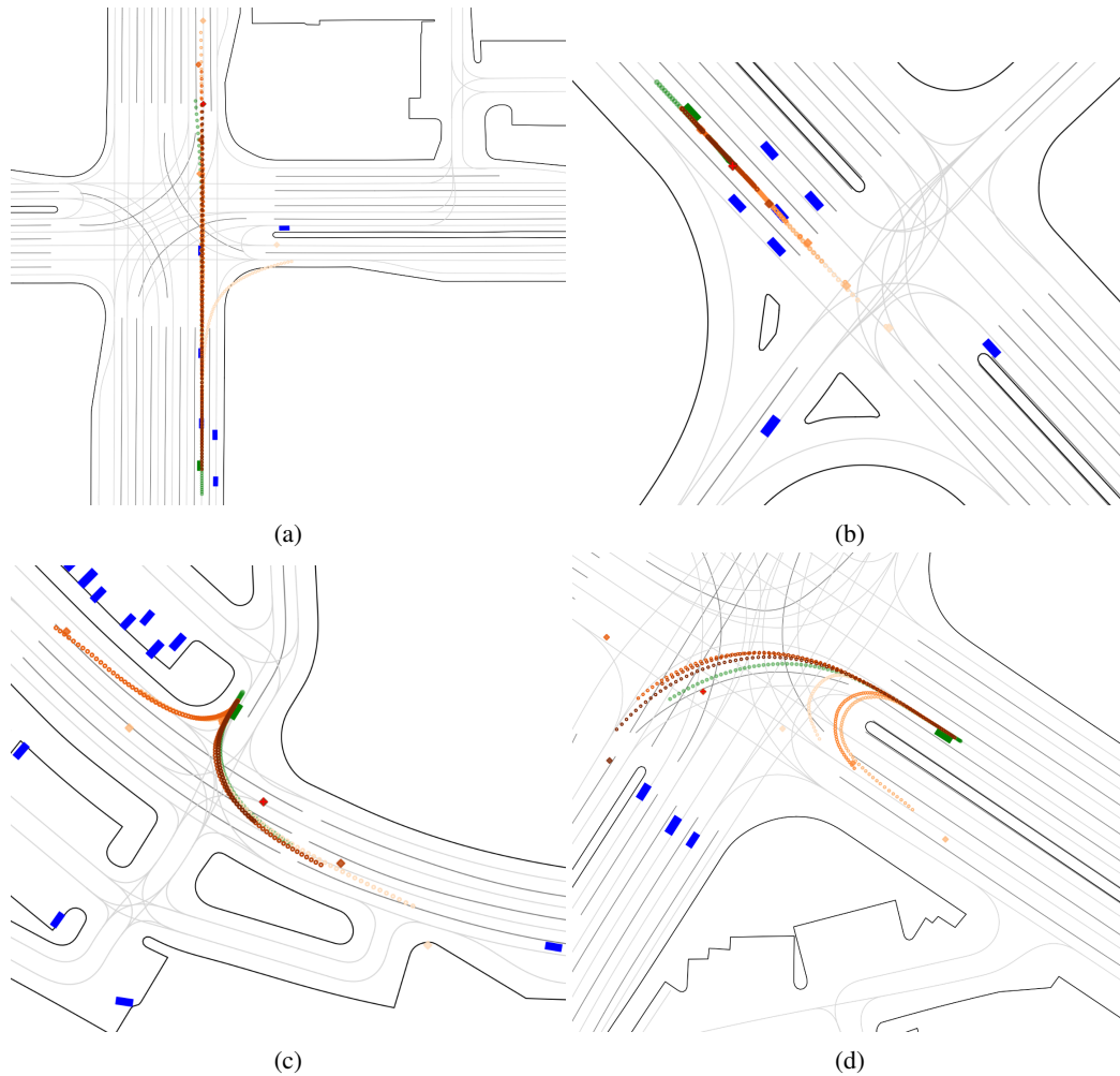
Figure 6: The qualitative results of motion prediction task in WOMD. The blue rectangles indicate the other traffic agents and the green one is the vehicle to predict. The green dots compose the ground truth trajectory containing both the history frames and the future. The rhombus marks represent the proposals and we use the intensity of colors to indicate the degree of confidence predicted by STR. Correspondingly, each predicted trajectory for each modality is shown in a sequence of dots with the same color as its proposal. The red cross symbol is the ground truth static proposal.
