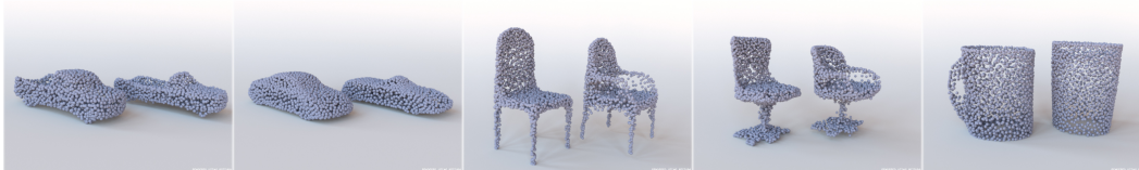
Figure 8: Editing parts in point clouds using vector arithmetic on the AE latent space. Left to right: tuning the appearance of cars towards the shape of convertibles, adding armrests to chairs, removing handle from mug.
