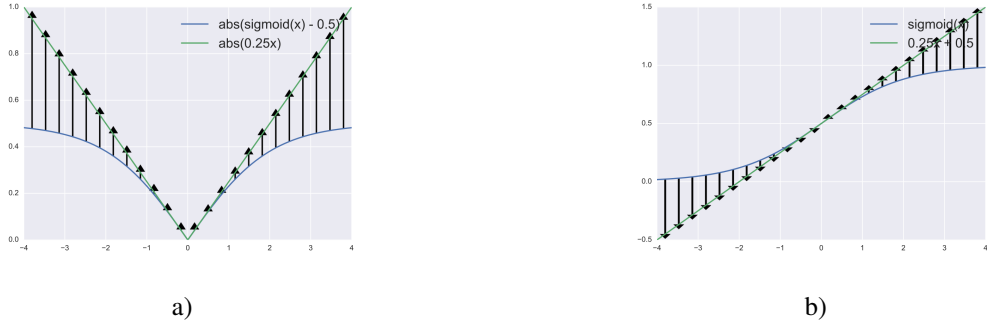
Figure 3: The figures show how to evolve the model to make it closer to a linear network. Arrows denote the direction of the noise pushing the activation function towards the linear function. a) The quasi-convex envelope established by a |\text{sigmoid}(\cdot)| around |0.25x| . b) A depiction of how the noise pushes the sigmoid to become a linear function.
