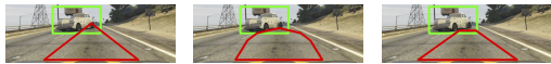
Figure 3. Three shapes of the danger zone. From left: triangle, polygon with 7 sides, and trapezoid.
