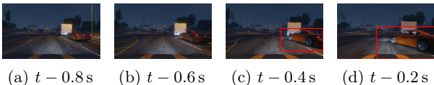
Figure 1. We show 4 images taken before the accident which happens at time t . From left to right, the estimated collision probability for each image is 0.00, 0.45, 0.99 and 1.00. Our algorithm successfully predicts the vehicle collision from these images. See (Lee et al., 2017) for similar demo videos.
