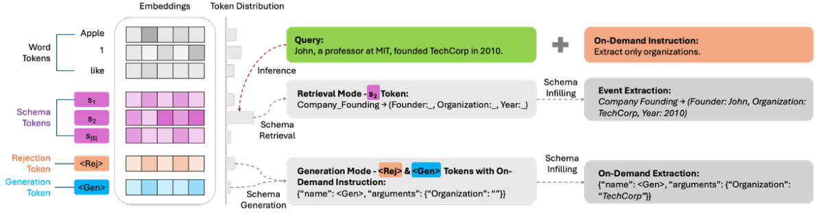
Figure 2: Overview of our proposed Schema as Parameterized Tools (SPT) framework. Schema-token embeddings are appended to the language model head as regular word tokens. The inference procedure consists of Schema Retrieval, Schema Generation, and Schema Infilling, which demonstrates a dual-mode extraction with Retrieval Mode and Generation Mode.
